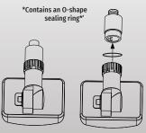
4. Tighten the sensor lock-ring
